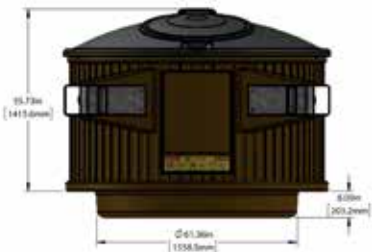
4.5YD SURFACE MOUNTED SHOWN WITHOUT CONCRETE RING
